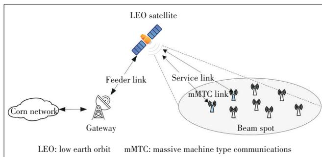
▲ Figure 1. mMTC system over LEO satellite
