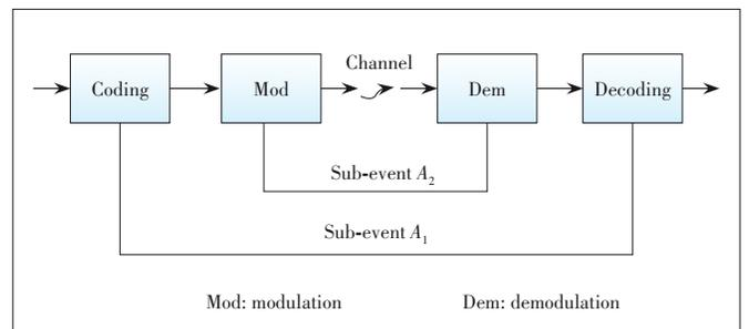
▲ **Figure 1. Current wireless transmission link**
