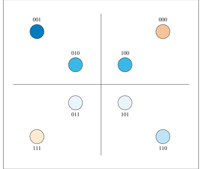
▲ **Figure 3. Error-corrected modulation constellation of (3, 1) coding**
