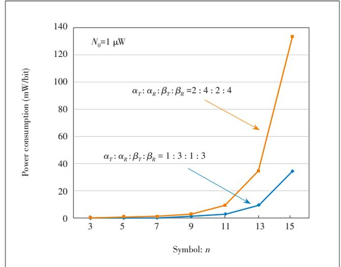
▲ Figure 4. Power consumption of event A under different parameters
