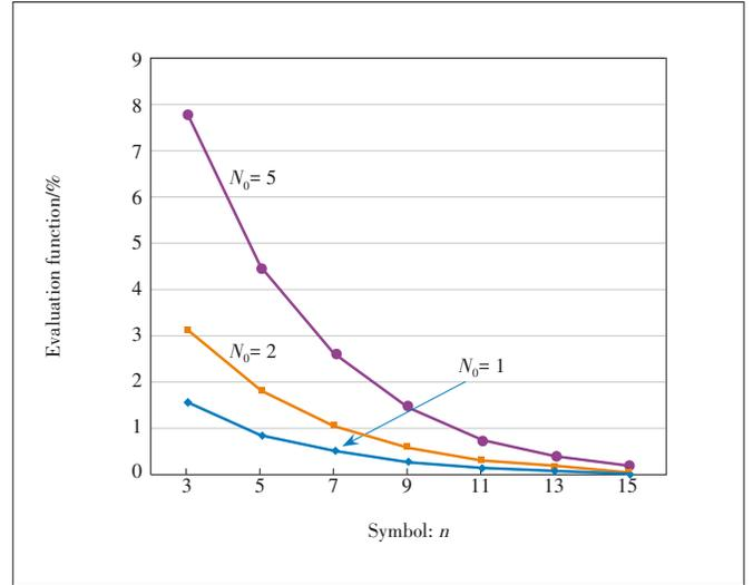
▲ **Figure 7.** Energy-saving evaluation function of the proposed modulation mode
